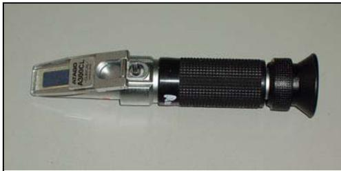
A refractometer tests for the concentration of the urine.
